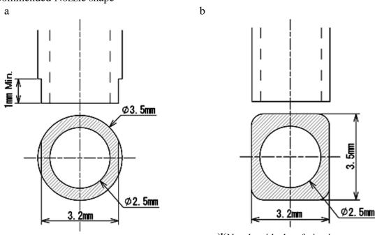
\*Nozzle with chamfering is recommended
