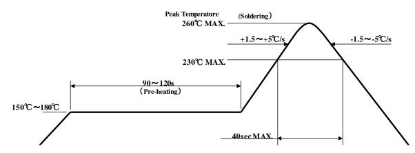
Note 1 Temperature Profile for the reflow should be set to the surface temperature of resin which is on the of LED. This should be the maximum temperature for soldering. Lowering the heating temperature and decreasing heating time is very effective in achieving higher reliability.
