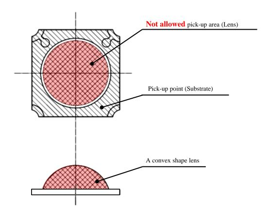
Please adjust the load, pick-up point, nozzle diameter, etc. before mounting because over load can cause breakage of the product.
