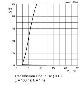
Fig. 3. Dynamic resistance with positive clamping voltage; typical values
