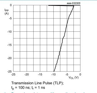
Fig. 4. Dynamic resistance with negative clamping voltage; typical values
