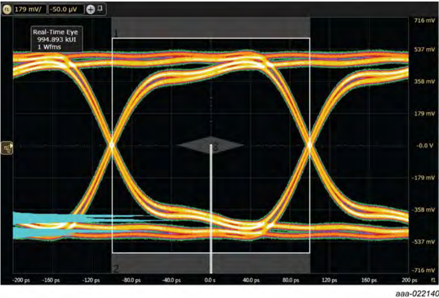
Fig 7. USB 3.1 eye diagram, test board with PCMF2USB30; typical values
