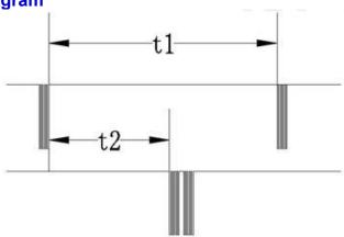
Note: When the op code is 0x01, T1  $\geq$  250ms; T2 = 200  $\sim$  210ms.
