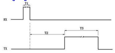
Note: For processed output: T1 = 0.1-5ms; T2  $\geq$  75ms; T3 = 0.6-65ms For live output: T1 = 0.1-10ms; T2 = 4.5-6.0ms; T3 = 0.55-65ms
