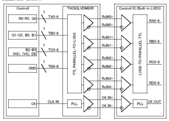
When using "6-bit Transmitter", please connect the unused channel of the control IC receiver as described in the diagram below.
