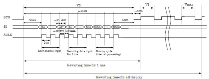
3 lines (SCS, SCLK, and SI) are control signals to rewrite.
