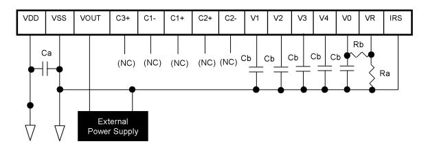
Ca: 1.0 to 4.7uF (Voltage rating 定格電圧: 10 to 35V)
