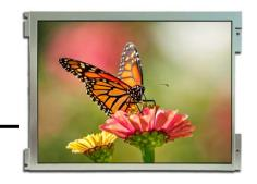
Kyocera offers two versions of 10.4" VGA TFT LCDs: the AN00 is the normal brightness version with 400nits brightness and the AN20 is the same panel but with the CCC (constant current circuit) built-in. Both products feature long life LED with 70K hours lifetime, wide operating temperature range and standard CMOS interface.
