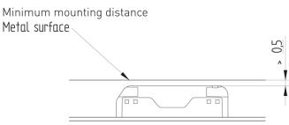
Compliance with creepage distances and clearances has to be ensured by the structural design of the luminaire.
