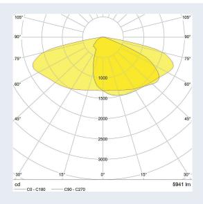
Light distribution: IESNA Type 4 Medium measured with Philips Fortimo Fast Flex LED 2x6 DA HE
