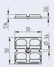
Height 7.14 mm Width 50 mm50 mm Length Type of fixing Screw fixing: (0.5 Nm) screws M3 LED Type Philips Fortimo Fast Flex LED 2x6 DA HE and LED modules with 12.5 mm pitch according to Zhaga Book 15 12.5 mm Pitch distance PMMA Material Colour clear Lense surface High gloss Permissible application temperature -40 °C up to +80 °C
