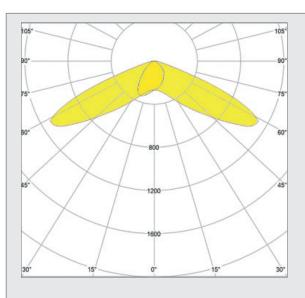
Light distribution: IESNA Typ 1-short measured with Philips Fortimo FastFlex LED 4x16 DHE G4
