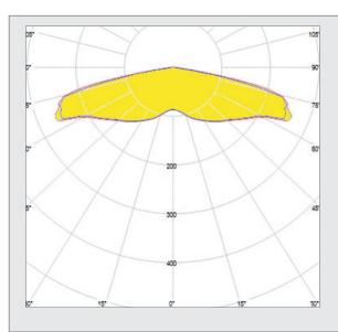
Light distribution: IESNA Typ 5-sqare measured with Philips Fortimo FastFlex LED 4x8up PR G5
