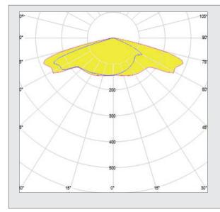
Light distribution: IESNA Typ 4-medium measured with Philips Fortimo FastFlex LED 4x8up PR G5
