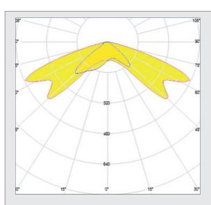
Light distribution: IESNA Typ 2-short measured with Philips Fortimo FastFlex LED 4x8up PR G5
