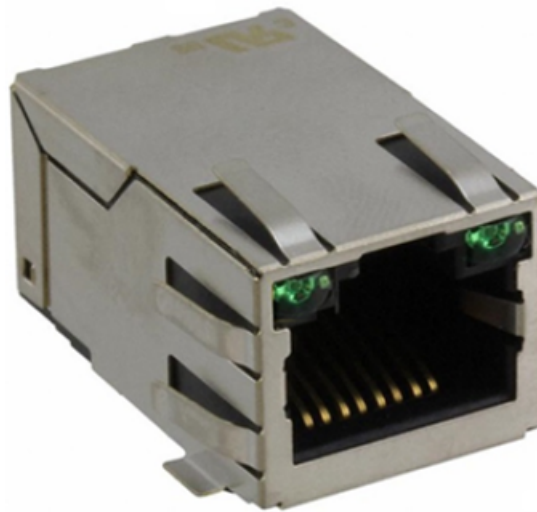
Figure 16: VCU129 Ethernet PHY Status LEDs
