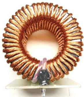
Figure 22. Synchronous Boost Inductor
