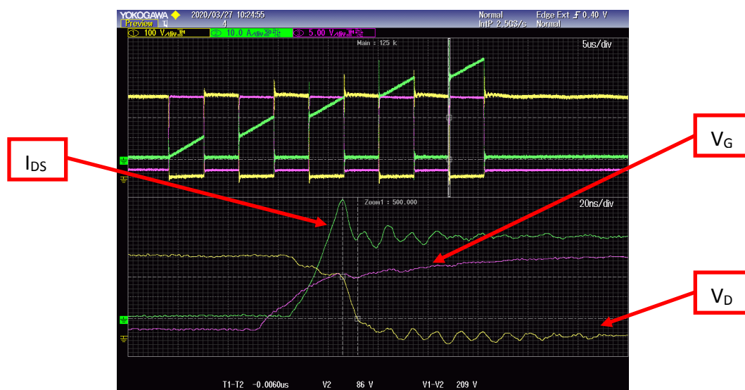
Figure 25. Double pulse waveforms
