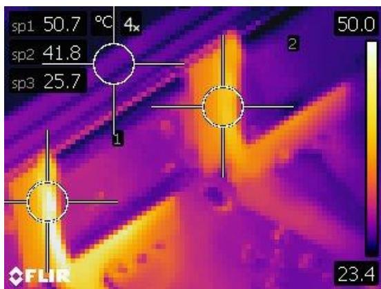
Figure 24. Thermal Scan of MOSFET (650V)
