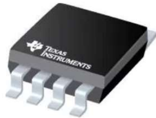
Figure 4: Cree's Flyback controller IC (P/N: UCC28740) from Texas Instruments Inc.
