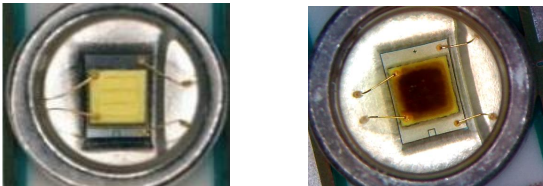
Figure 6: Examples of normal (left) and VOC degraded LED (right)
