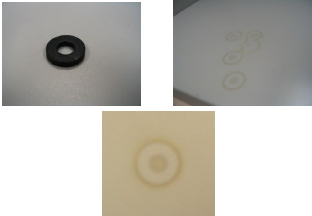
Figure 9: Evidence of VOC outgassing from an O-ring
