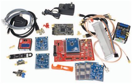
This starter pack extends the Level 1 pack by adding the features needed for working with external targets (besides the included UFO targets). The advanced breakout board can perform level-shifting when you aren't working with 3.3V I/O or need additional breakout.
