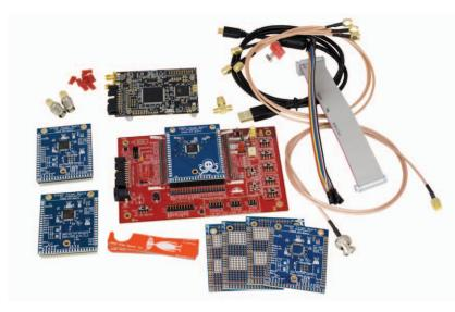
This starter pack is great for getting involved with side-channel power analysis and fault injection attacks. It includes our ChipWhisperer-Lite Capture and our versatile UFO board.
