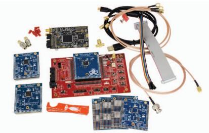
This starter pack is great for getting involved with side-channel power analysis and fault injection attacks. It includes our ChipWhisperer-Lite Capture and our versatile UFO board.
