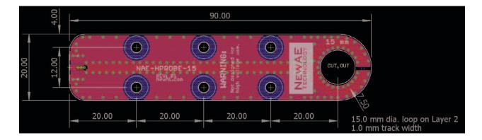
The above shows all four layers of the PCB used in the planar H-Field probe. The specific layers are shown on the following page.
