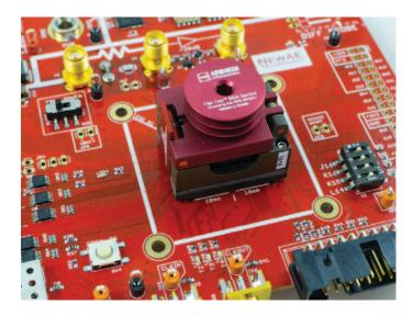
The socket can fit any Artix 7 device in the FT256/FTG256 package. Currently this means the following devices are supported: XC7A15T, XC7A35T, XC7A50T, XC7A75T, XC7A100T. If ordering an FPGA for the socket ensure it is in the FT256/FTG256 package. Note the 'G' package indicates usage of lead-free (Sn/Ag/Cu) solder balls, whereas the FT256 package uses Sn/Pb solder balls. Either walls will work with the BGA socket.
