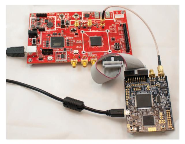
The CW305 can be used with the ChipWhisperer Capture hardware (either CW1173 or CW1200). The Chip-Whisperer capture hardware provides power analysis, along with clock and voltage glitching. This forms a complete low-cost and standalone lab that does not require any additional test equipment such as oscillo-scopes or power supplies.
