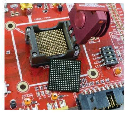
When closed, the socket has a heat sink on top of the FPGA. Note the socket prevents usage with an EM probe or similar.
