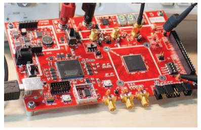
The CW305 is an advanced target for performing power analysis & fault injection attacks against hardware cryptographic functions implemented in FPGAs.
