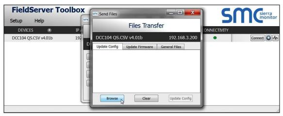
• Once download is complete, click the Restart Button (or simply cycle power to the QuickServer) to put the new file into operation. Note that it is possible to do multiple downloads to the QuickServer before resetting it.
