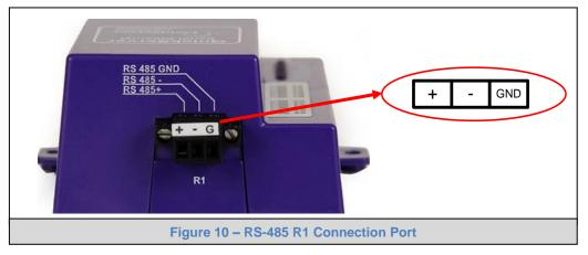
The following Baud Rates are supported on the R1 Port: 110, 300, 600, 1200, 2400, 4800, 9600, 19200, 20833, 28800, 38400, 57600, 76800, 115200
