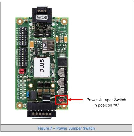
The QuickServer Carrier Board power jumper is set to position A by default, but can be changed to position B for other power supply requirements.
