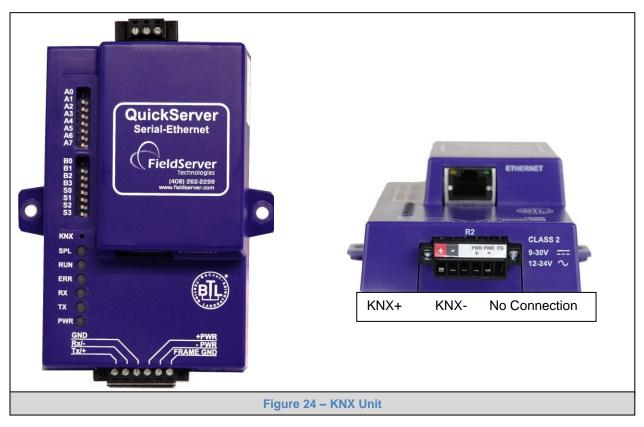
The KNX Connector consist of a KNX + and KNX- terminal. Each terminal corresponds to the red KNX+ and gray KNX- bus connections on a KNX bus.
