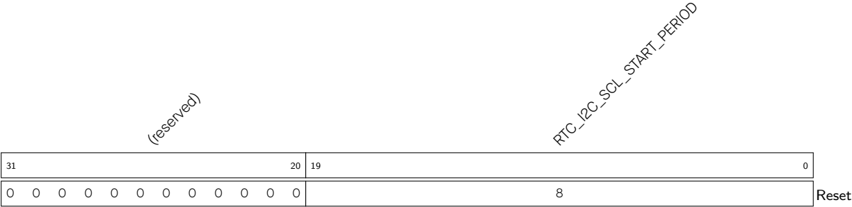
Register 1.17: RTC_I2C_SCL_START_PERIOD_REG (0x001C)
