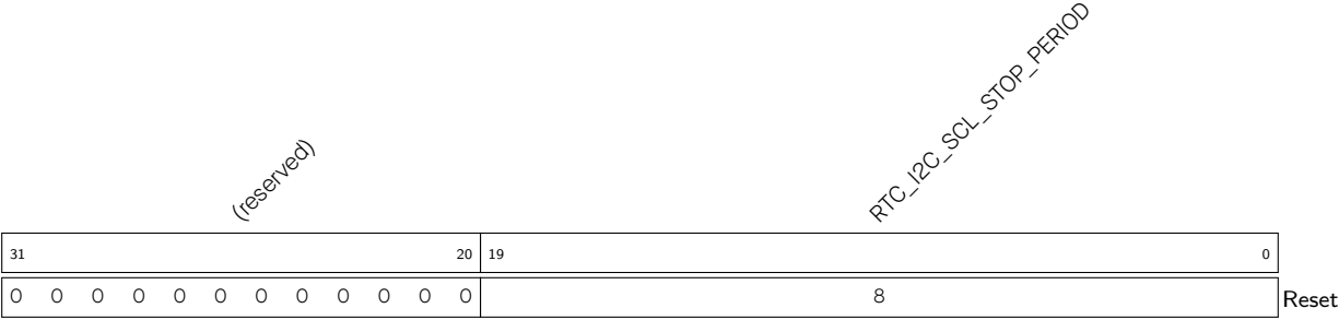
Register 1.18: RTC_I2C_SCL_STOP_PERIOD_REG (0x0020)
