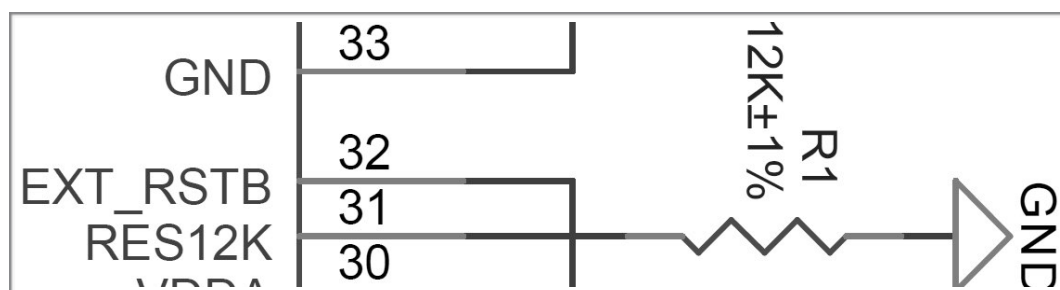
Figure 1-9. ESP8266EX External Resistor
