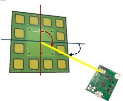
The full system is made of anchor units positioned in line-of-sight manner from tag units. The Tag Board is regularly transmitting a specific localization advertising signal. The Anchor Board integrating an Antenna array at the other side of the communication link is providing phase, which leads to angle information. The position of tagged items is calculated by triangulation from different anchors.
