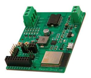
Specially designed console firmware as well as example code can be downloaded to get started quickly and easily. The code is well documented and open source and is based on the well-established ESP-EDF framework and RTOS. SwarmDrive can be used as a starting point for getting insight into the inner workings of algorithms for driving a motor.
