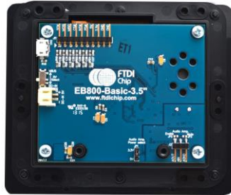
Figure 3-1 – VM800B module profile 3.5” display version
