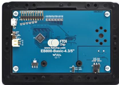
Figure 3-2 - VM800B module profile 4.3” display version
