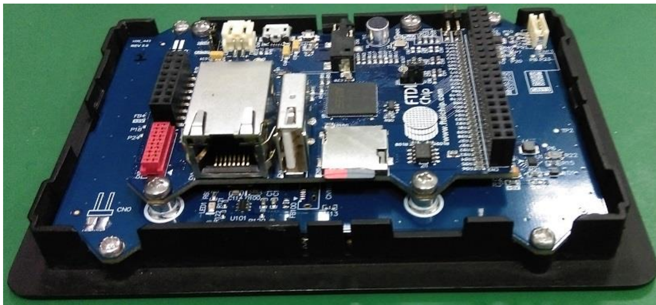
Figure 7-1 – ME812A-WH50R connects to MM900EV1A Module
