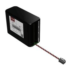
Type DSM Standard Supercapacitor Modules provide a wide range of capacitance values and voltages to enable simple, rapid implementation into any system. Each module features an insulated construction with integrated cell balancing, cable assembly with a Molex Mini-Lock connector, and 85°C rated supercapacitor cells.
