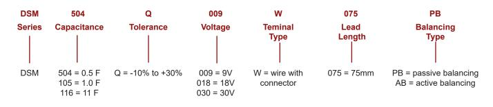
Type DSM, Standard Supercapacitor Modules Knowles
