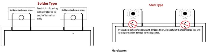
Hardware: M6≈1/4-20 stud / bolt Copper flat washer, M6 washer with 12 mm (0.472") OD
