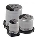
Type AVES Capacitors are rated for 1000 hours at 105 °C with low impedance characteristics. They are ideal for high density PC board packaging. The Type AVES offers a low in-place-cost for a high quality performer. The vertical cylindrical cases facilitate automatic mounting and reflow soldering into the same footprint of like-rated tantalum capacitors except without the need for voltage derating.
