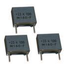
The Type 160 series radial lead metallized polyester box capacitors are constructed in rugged rectangular plastic cases with lead spacings that are standard in the electronics industry. All Type 160 capacitors are available in bulk with a .217"±.039" lead length, and they are good for general purpose applications such as bypass, decoupling, energy storage/discharge and arc suppression.
