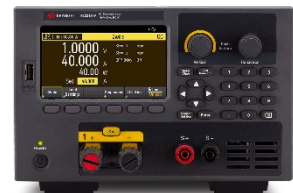
Figure 1. EL33133A 250 W bench electronic load 150 V, 40 A
