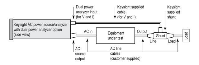
**Figure 1**. Test configuration of efficiency measurement using an Keysight AC source with the 020 dual power analyzer option
