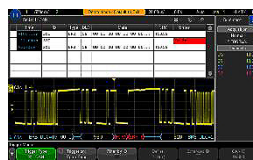
Figure 17. CAN-FD decode and trigger.
