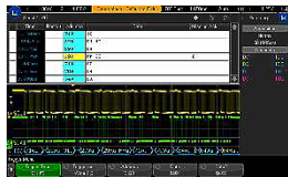
Figure 15. I2C decode and trigger.
