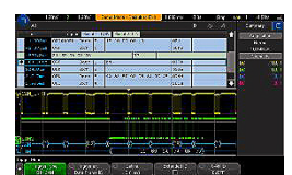
Figure 19. Multi-bus time aligned decode.
