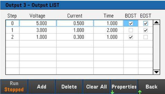
Figure 8. Output sequencing and Output LIST mode setting
