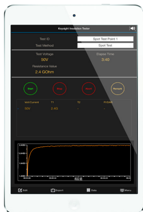
Figure 2. Perform remote testing with Keysight InsulationTester Application
