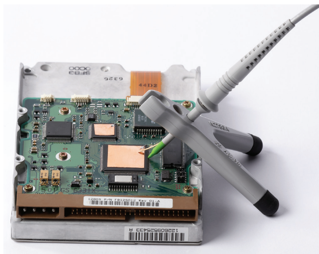
Figure 8. An IC cap adapter and ground blade with optional N2876A two-leg probe positioner offers an ideal hands-free solution for short circuit-proof probing of a fine-pitch IC. The N2877A deluxe accessory kit and N2878A fine-pitch accessory kit contain one N2876A two-leg probe positioner.
