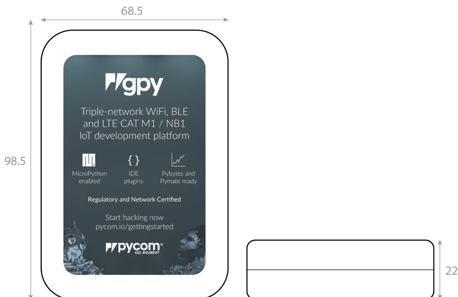
Figure 8 – Mechanical drawing of packaging – Units: mm
