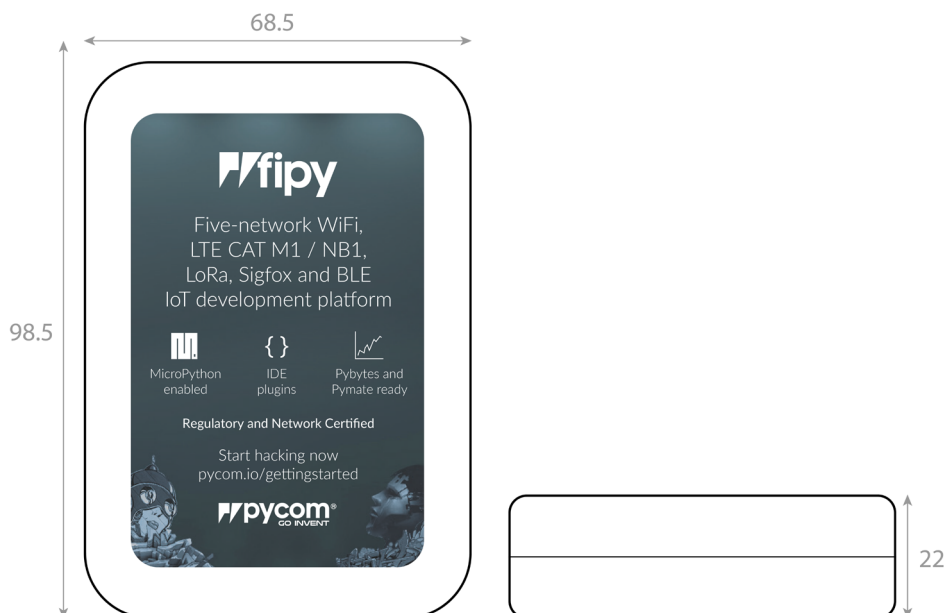
Figure 7 – Mechanical drawing of packaging – Units: mm
