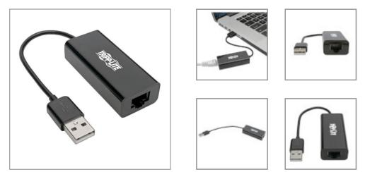
Connects your USB-enabled computer or laptop to a 10/100 Mbps Ethernet network without installing an internal Ethernet card.
