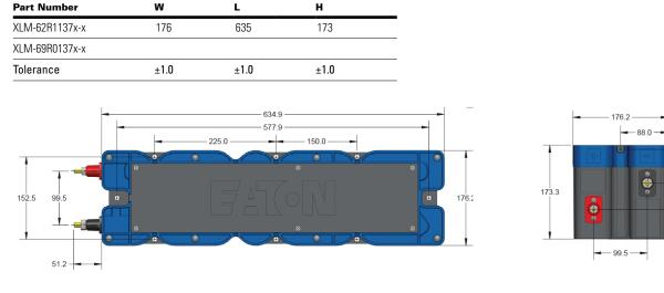
Positive Terminal: 5/16" – 18 threaded stud Negative Terminal: 3/8" – 16 threaded stud
