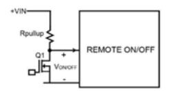
Logic type active mode: DC/DC ON : Q1 OFF
