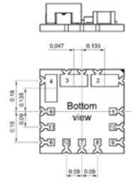
Pad  $1\&5\sim12=0.118"\times0.059"$ Pad  $2\&4=0.17"\times0.08"$ Pad  $3=0.168"\times0.08"$
