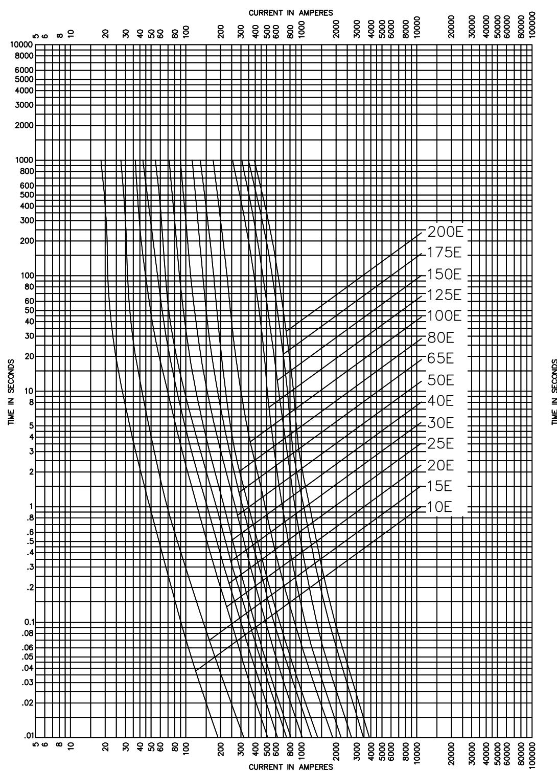
15.5 to 17.5 kV time-current curves — total clearing
